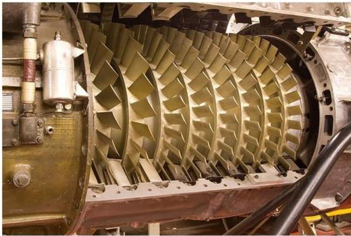
**Figura 6 – Compressor Axial.**
